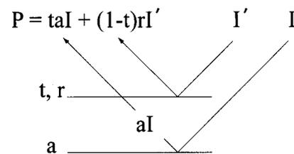
Fig. 2. Optic array describing the episcotister luminance model. Note that the background is illuminated only directly and not through the layer.
